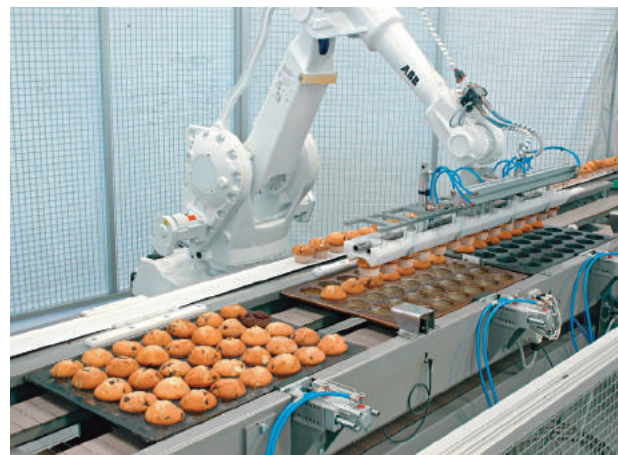
Figur 14.3 Roboter lager muffins. Foto: ABB.
